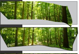
Insert the first three flex holders on the sides and the top edge and engage into the first or second tooth of the profile. When inserting each flex holder pull the fabric firmly away from the starting point in order to prevent wrinkles.
